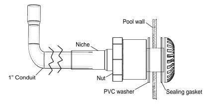
GloBrite Light Niche (Fiberglass pool) Installation Diagram
