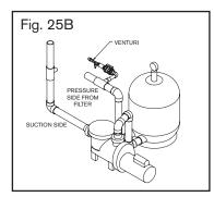
New Installation using Paramount venturi installation kit.
